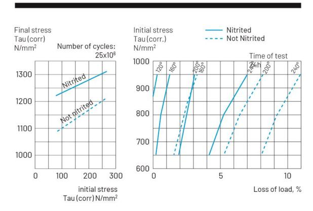
In diagram 1 the fatigue properties of this grade are illustrated in a Goodman-diagram, based on a special test spring design.
